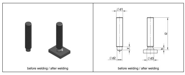
The threaded stud type RD is threaded almost to the top of the welding tip which is reduced to about the core diameter of the thread. Thus the fillet diameter will only be slightly (0,5-1 mm) bigger than the external diameter of the thread. It is worthy of note that the reduction of the welding tip diminishes the bearing force of the stud by approximately 15% in comparison to the type MPF/PD/FD. Thus - if necessary - the next bigger diameter should be chosen.
