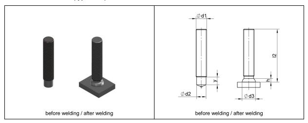
The threaded stud type MPF is threaded to approximately the top of the welding tip. The diameter of the unthreaded stud section on the welding tip corresponds to the pitch diameter of the thread. Thus the diameter of the weld-fillet is approximately 3-4 mm larger than the external diameter of the thread.
